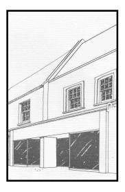
Left: Lack of stall risers at ground floor level resulting in an unbalanced shop front
